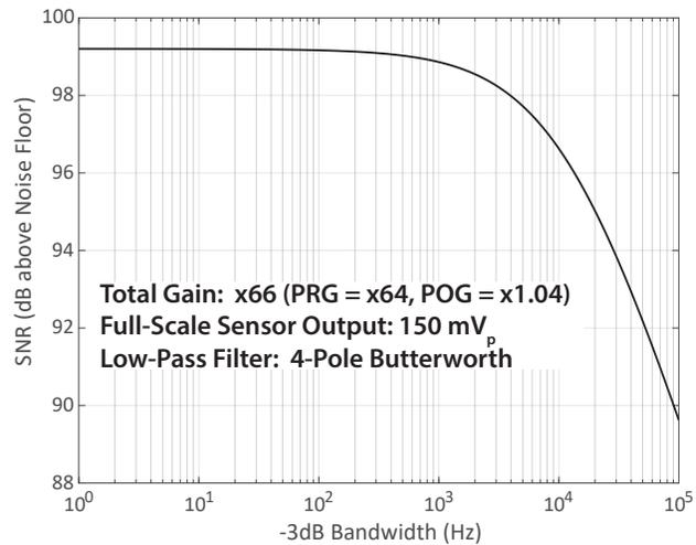
Figure 3) Estimated SNR vs. bandwidth for the setup in Figure 1A. The desired full-scale circuit output for A/D conversion is  $10 V_p$ .
