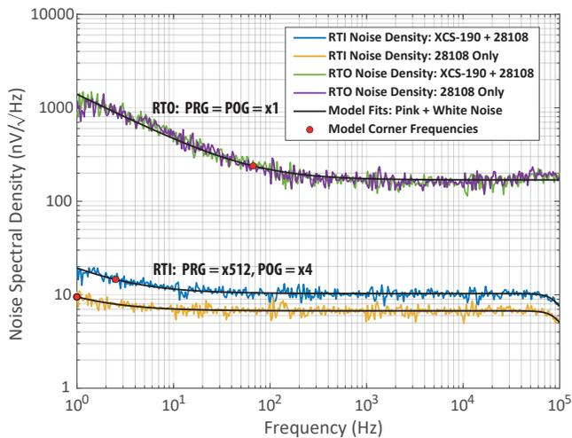
Figure 2) Measured noise spectral densities (see Figure 1A for setup) with model fits. See text for detailed discussion.
